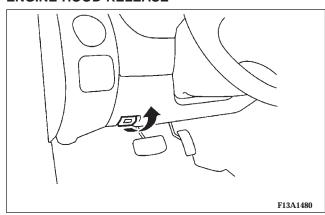
The engine hood release lever (located under the instrument panel near the driver's door) is used to unlock the engine hood.
